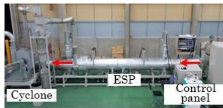
Figure 12. Prototype ESP-C (ESP: 400 mm O.D., 4400 mm Length)
